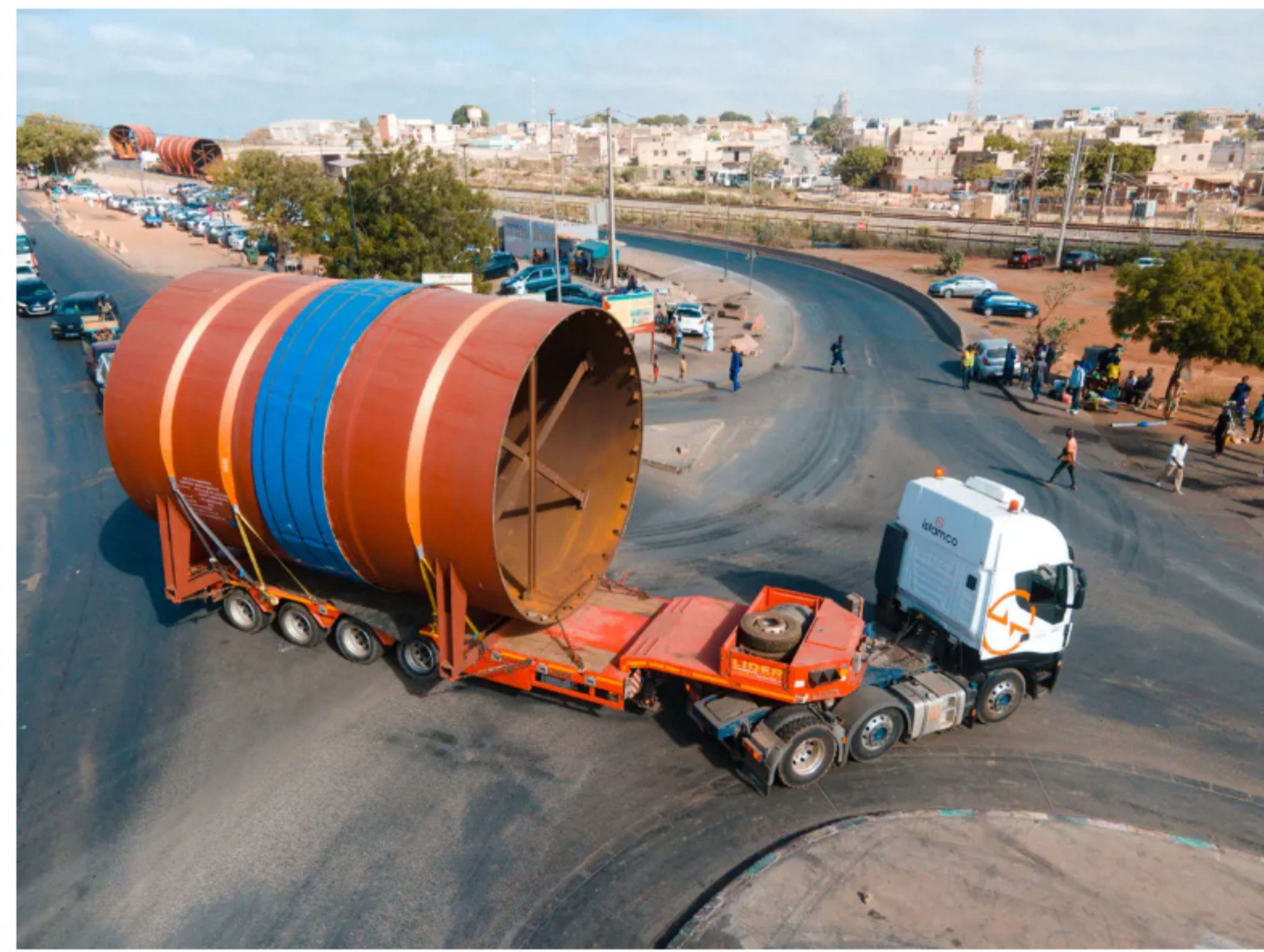
80% of the total cargo volume had to be delivered by the end of 2023. The first 656-ton critical shipment from China required special heavy lift expertise and significant infrastructure modifications, as four pedestrian bridges had to be removed for the eight 82-ton heavy kiln shells to pass safely en route to the building site.
